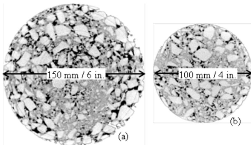
Figure: CT scan of asphalt column
